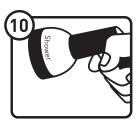
Set spray nozzle to "shower". Check for water accumulation at the surface of the jointing sand as a cue to stop watering. Wait until there is no free water at the surface of the joint and verify the depth of activation.
