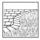
Complete your installation by back filling with topsoil, mulch or decorative stone over the EDGE BOND $^{\text{TM}}$  edging. This can be done as soon as your EDGE BOND $^{\text{TM}}$  installation is completed. EDGE BOND $^{\text{TM}}$  also offers a smooth surface that is paintable to blend into your hardscape projects.
